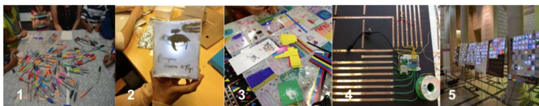
Figure 1. (1) Color pencils used for individual designs, (2) Single box prototype with LED light and decorative drawing, (3) Boxes mounted on the foam board, (4) Electric imp, copper tape connections, and LED matrix controller, and (5) Five boards connected to a mural with some LEDs turned on each board.
